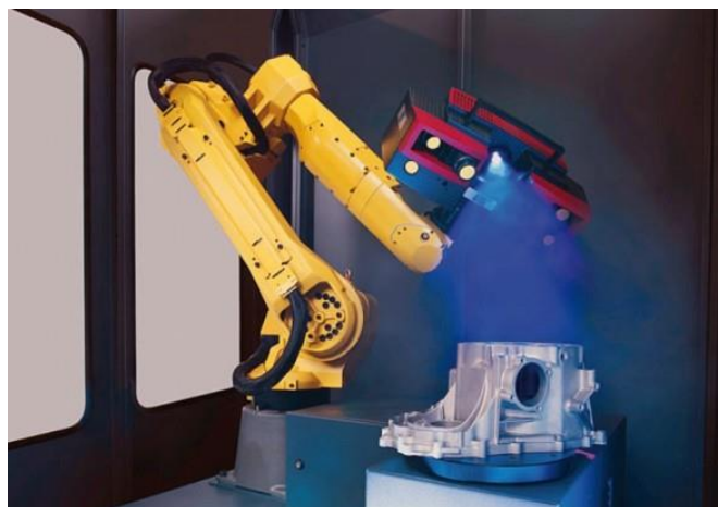
Obr. 8: Skener ATOS III Triple Scan [5]
