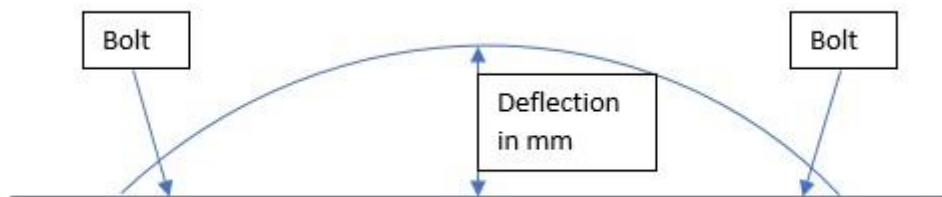
Figure 22 Mechanism of deflection in samples.
