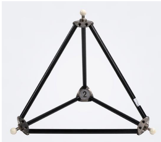
Obrázek 22: Tetrahedron TETRA-CHECK firmy Innovalia Metrology (14)
