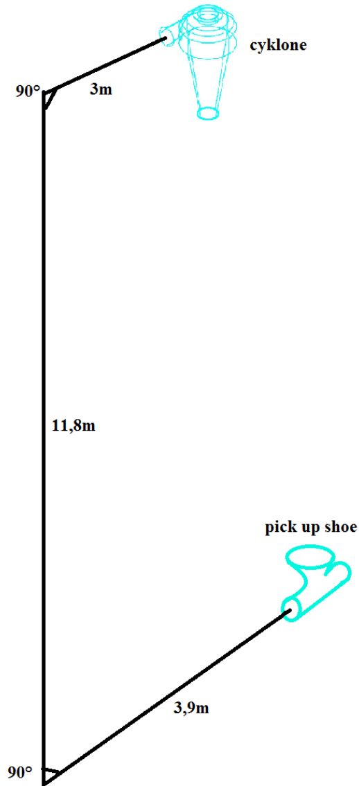
Figure 21 – the main line routing
