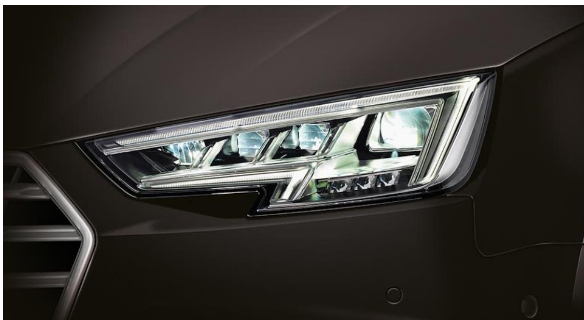
Obr. 1. Full LED světlomet Audi A4 s technologií matrix [25]
