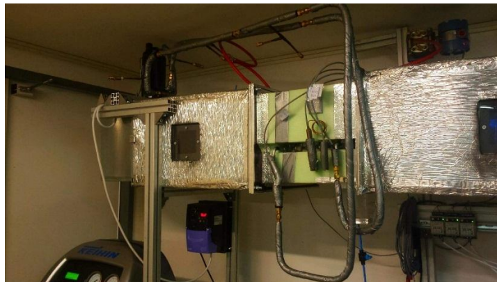
Fig. 26 Test rig with heat pump circuit
