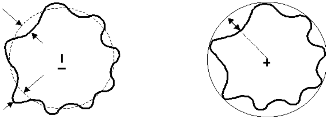
Obrázek 28: Least squares circle (LSC), (vlevo), Minimum circumscribed circle (MCC), (vpravo) [1]
