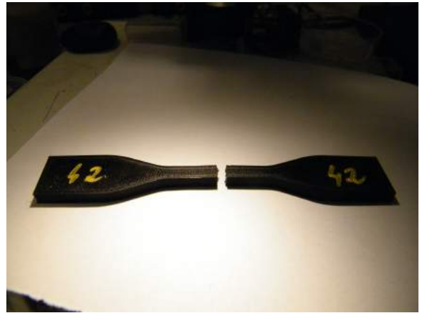
Figure 11.12: Straight break line of test specimen
