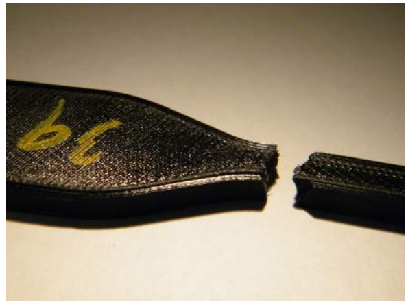
Figure 11.10: Delamination / separation of part shell from infill part
