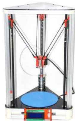
Figure 6.5: Delta FDM printer configuration
