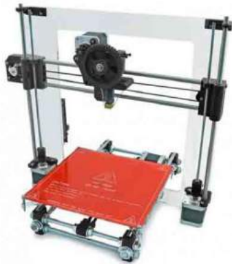
Figure 6.4: Typical 3-axis cartesian printer
