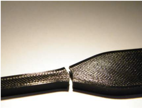
Figure 11.11: Test specimen broken outside of narrow region
