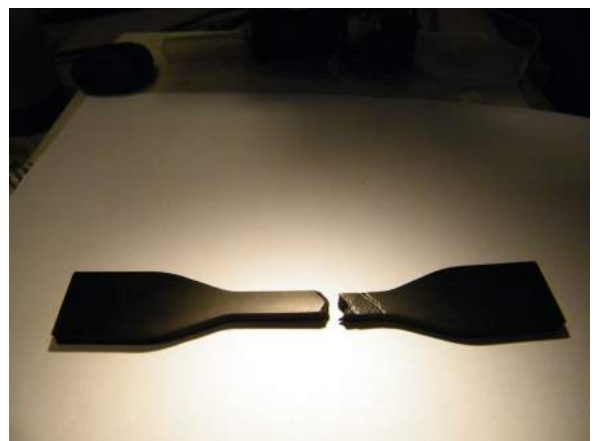
Figure 11.14: Test specimen, exhibiting plastic deformation
