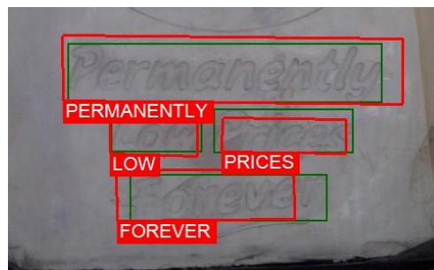
Figure 6.1 The proposed method detects and recognizes text in scene images at 10fps on an NVidia K80 GPU. Ground truth in green, model output in red. The image taken from the ICDAR 2013 dataset [53]
