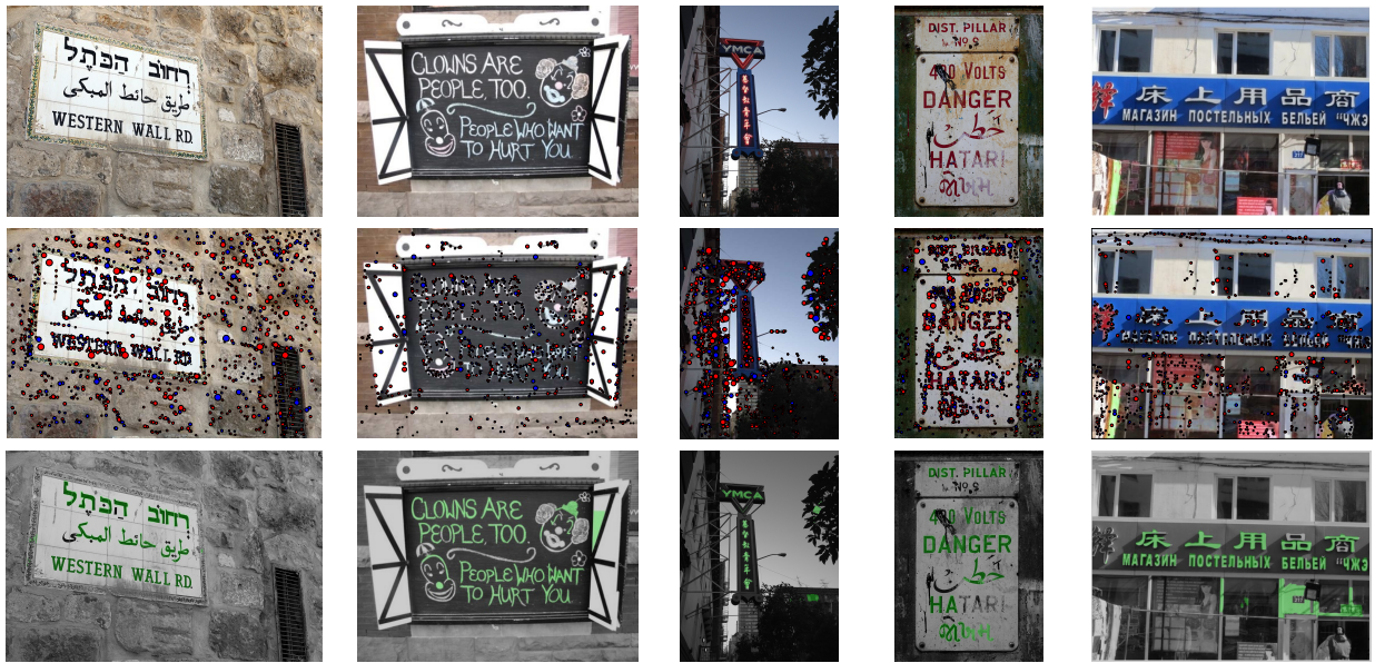
Figure 5.12 Scene text images with different scripts, fonts and orientations. Source images (top row), detected FASText keypoints (middle row) and resulting text segmentations (bottom row). Best viewed zoomed in color.
