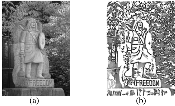
Figure 2.6 Stroke Width Transform (SWT). (a) the original image converted to grey-scale. (b) stroke width estimation for each pixel. Images taken from [29]
