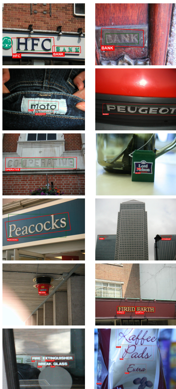
Figure 6.5 End-to-end scene text recognition samples from the ICDAR 2013 dataset. Model output in red, ground truth in green. Note that in some cases (e.g. top-right) text is correctly recognized even though the bounding IoU with the ground truth is less than 80%, which would be required by the text localization protocol [53]. Best viewed zoomed in color
