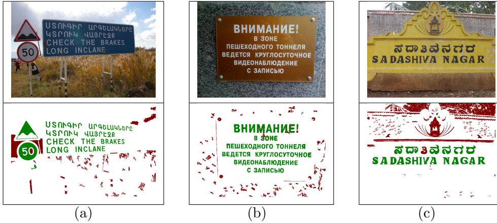
Figure 4.10 The features used by the sequential character classifier allow detection of characters in various scripts - Armenian (a), Russian (b) and Kannada (c). Note that the training set contains only Latin characters.
