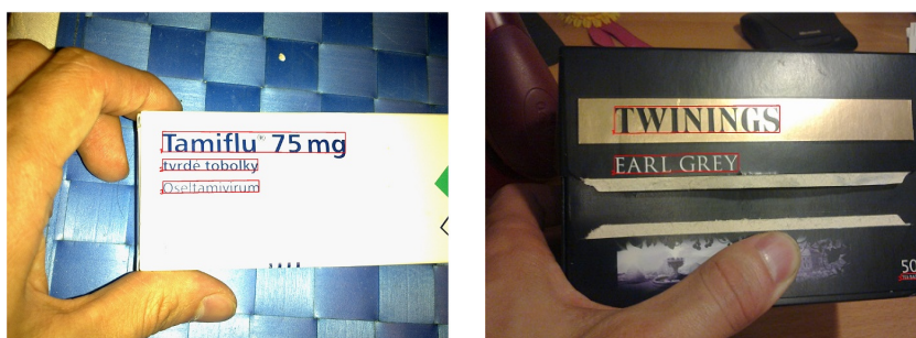
Figure 1.3 An aid for visually impaired people. Any detected text is automatically read out loud using a speech synthesizer
