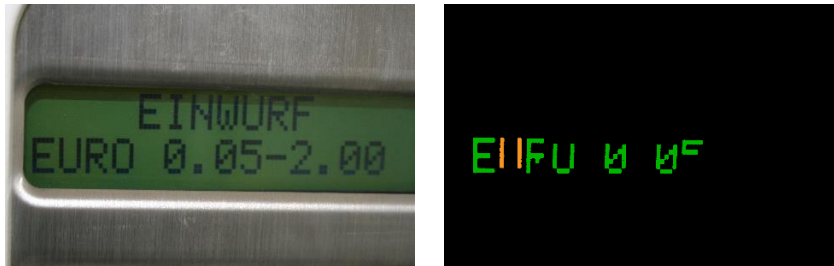
Figure 2.10 The text segmentation protocol [22] may not always provide good clues whether characters could be successfully processed by a subsequent OCR stage - source image (left) and sample segmentation output (right). Well-Segmented atoms in green, Broken atoms in orange
