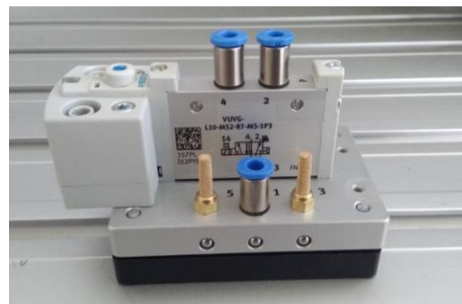
Figure 16: 5/2 Mono-stable solenoidal value
