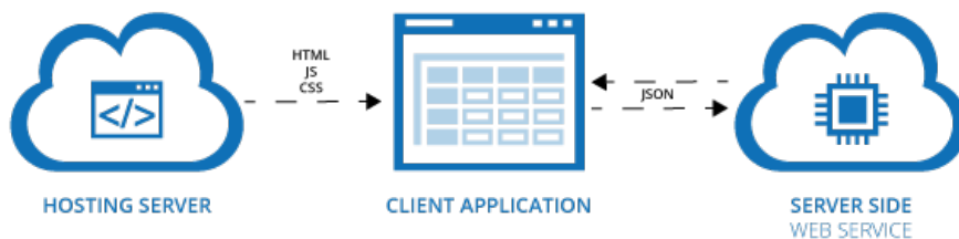
Figure 2.1: Diagram of service-oriented single-page web application.
