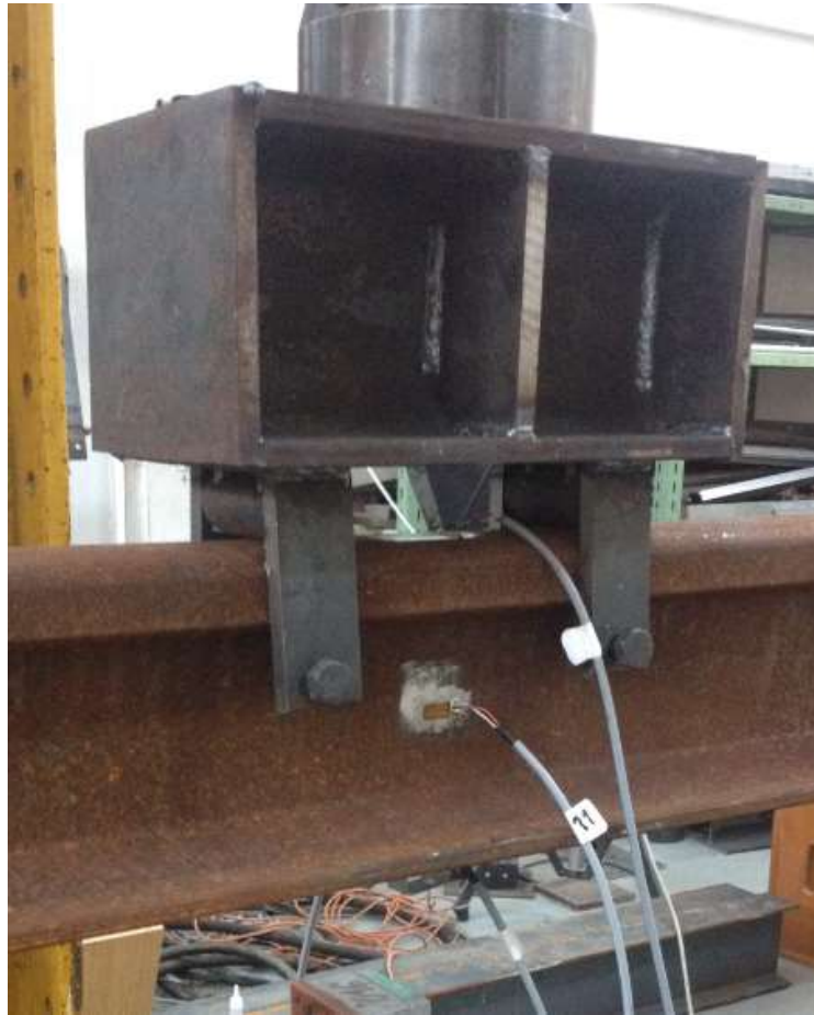
Figure 15. Load-application structure. Photo
