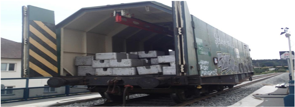
Figure 25: View of the wagon with uneven distribution of the additional mass
