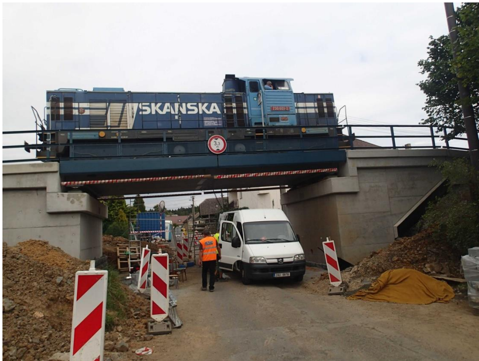
Figure 32: HV730 Test locomotive making a pass on the bridge
