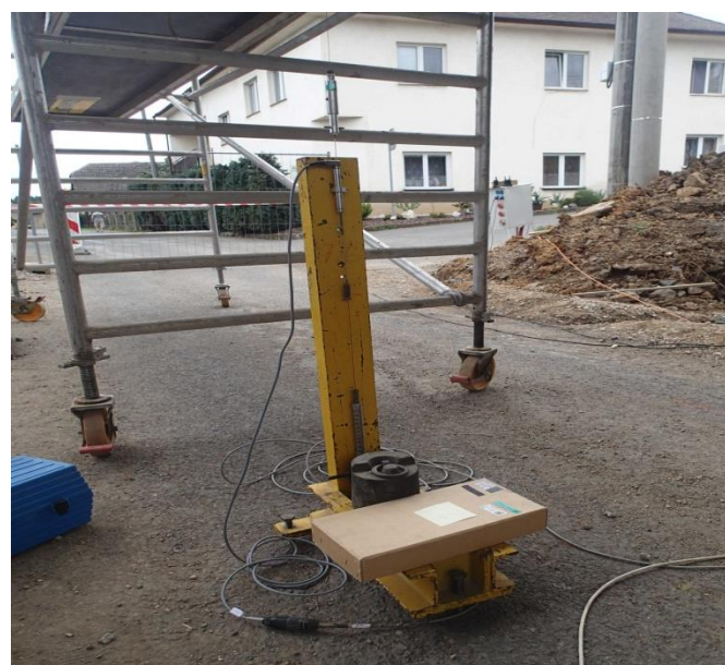
Figure 20: Inductive displacement sensor at mid-span
