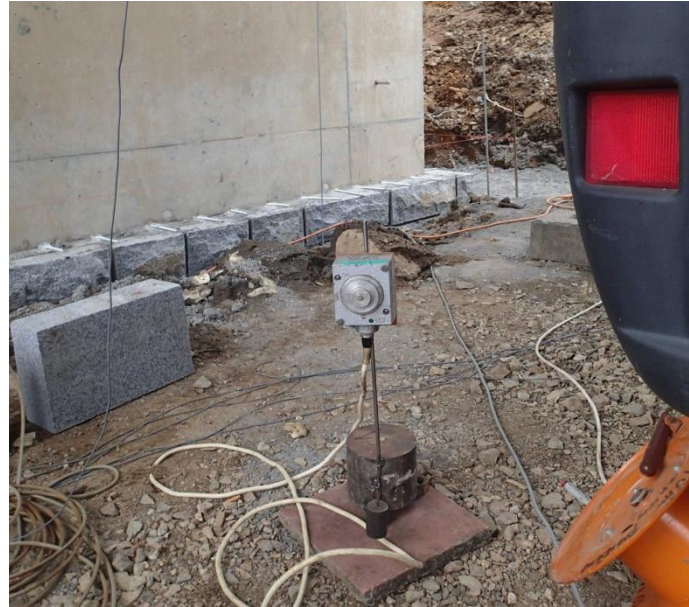
Figure 19: Potentiometric deflection sensor at quarter span
