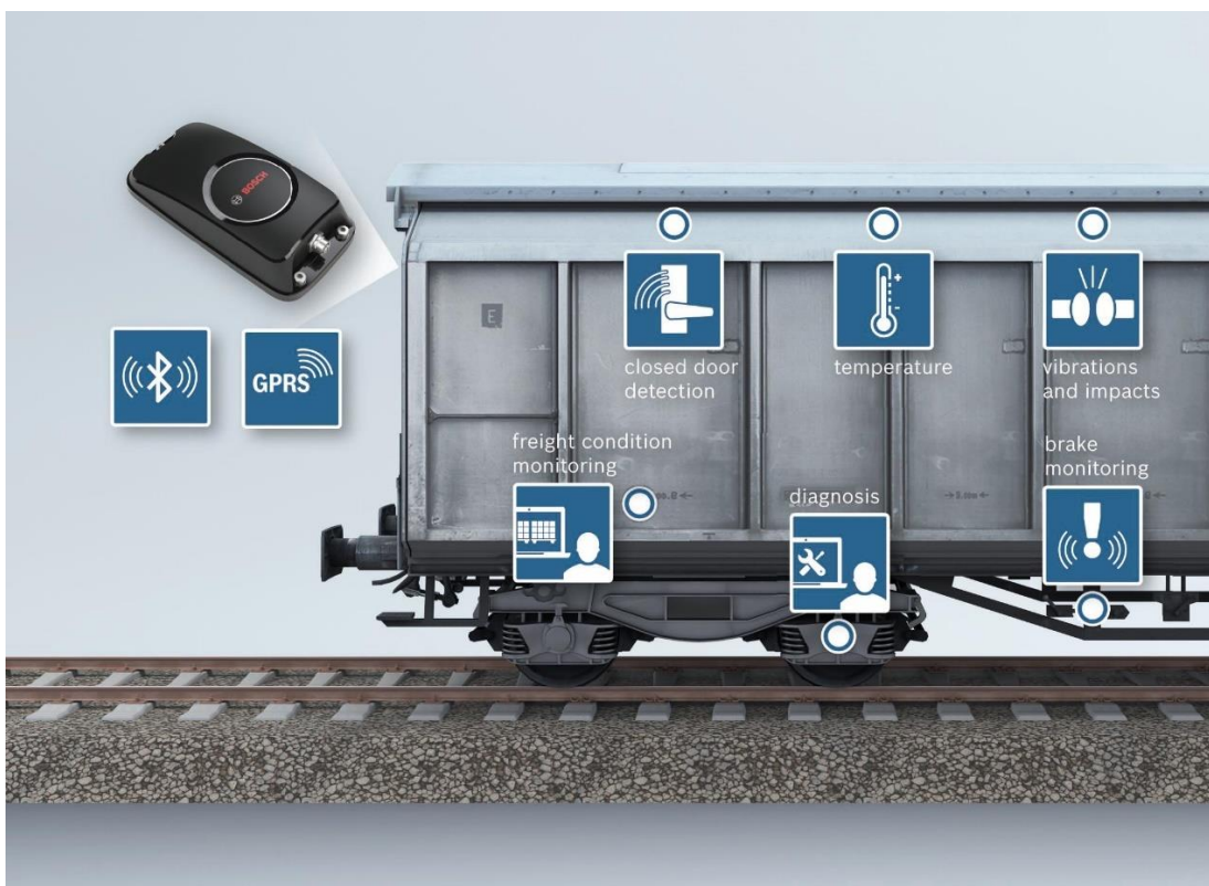
Figure 1: Bosch and SBB smart wagon concept. [3]
