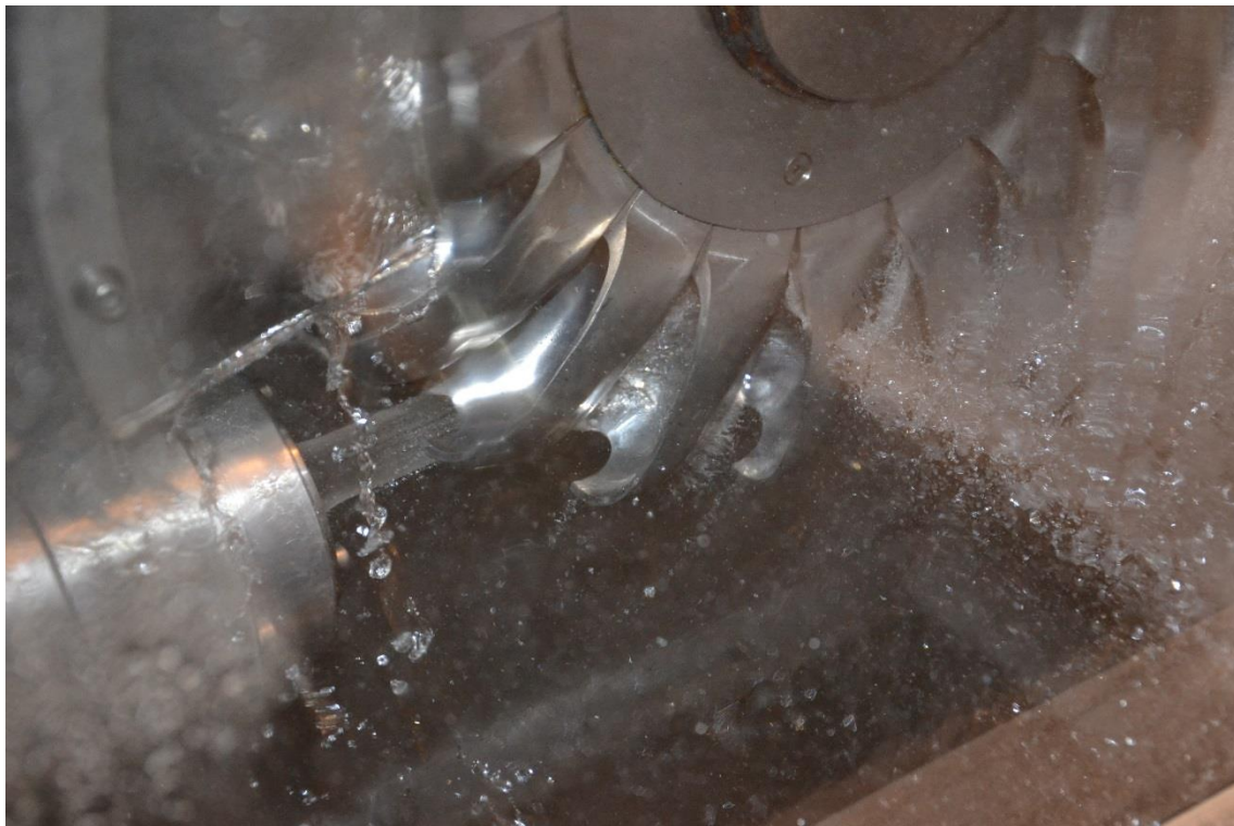
detail trysky: Q = 18,12 \text{ l/s} , 1200 \text{ ot/min}
