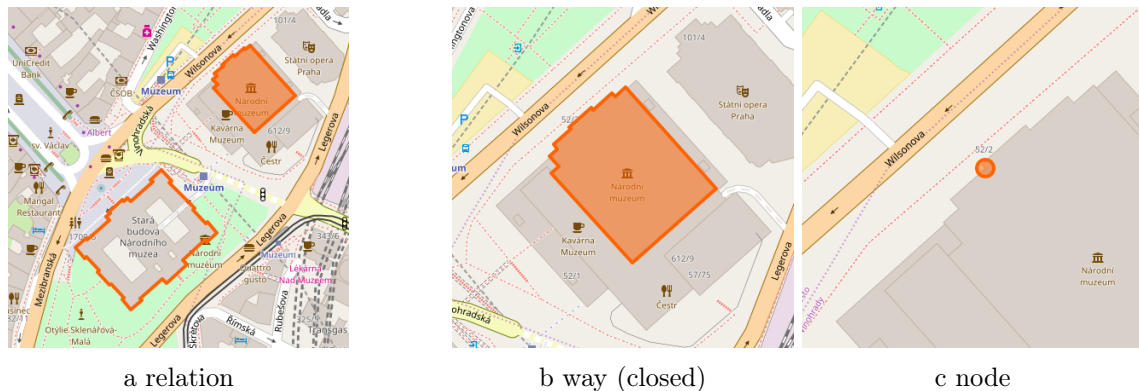
Figure 4.4: Types of objects in the OSM. The relation can contain ways , nodes but also other relations . A way is an ordered sequence of nodes and can be either closed (a polygon) or open. Each object may contain tags. Imagery obtained using [140]
