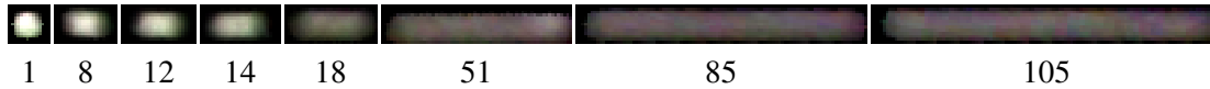
Figure 5.3. Object class representation of table tennis ball for 6 pixel radius. The top row show blurred appearances of the ball with different lengths (bottom row), which set the blurriness. The estimated percentage of the background was subtracted and only blurred object appearance is stored. The brightness of three longest blurred appearances was enhanced for better visualisation (producing some artefacts).
