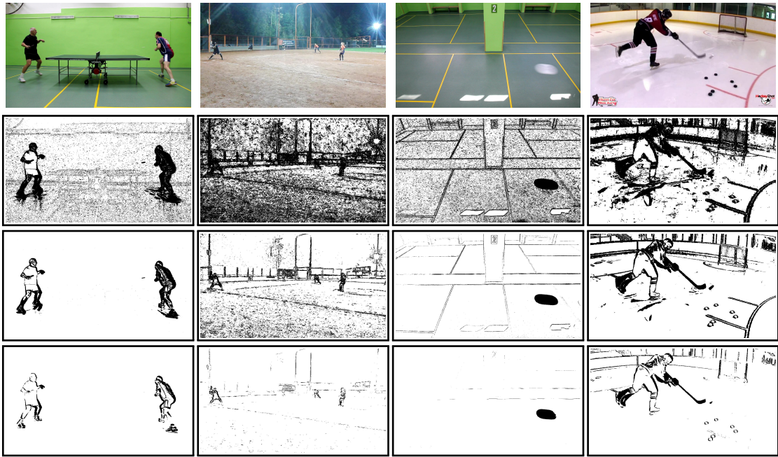
Figure 4.1. Selected frames from the FMOv2 dataset (top row) and binarised temporal difference images for thresholds (from second to bottom row) – 5, 25 and 50.
