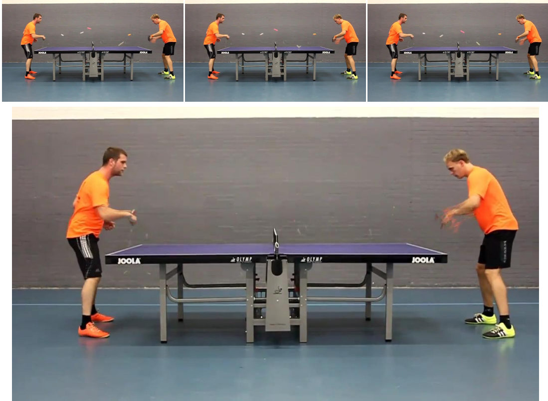
Figure 3.1. Example of the background estimation on a sequence with 5 table tennis balls that are FMOs. Median of 5 consecutive frames (3 of them are in the top row) gives the background B_t (the bottom image). The players are moving but their motion is not interpreted as FMO (see Algorithm 1).
