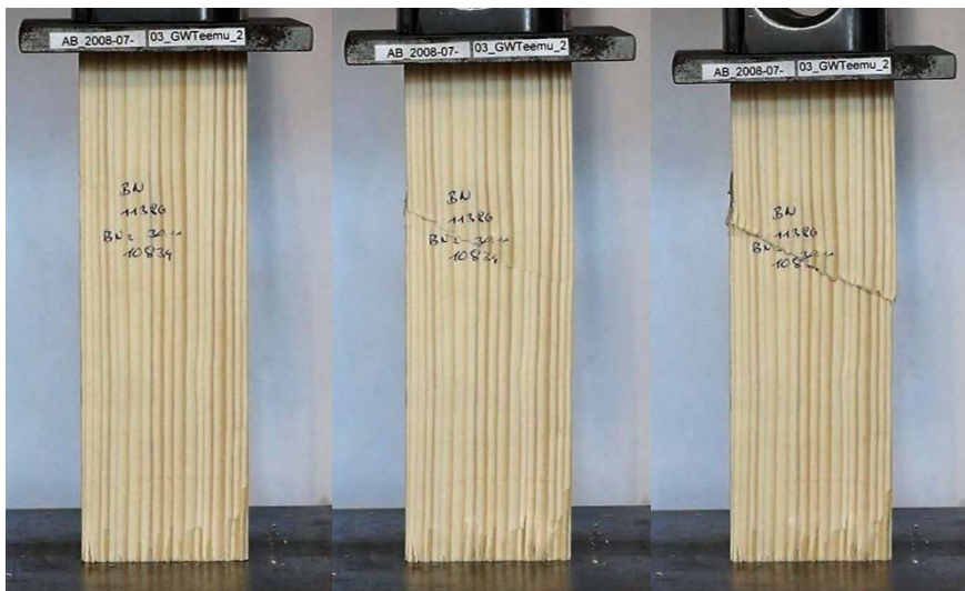
Photo 5-4 BN 0 compressive strength test
