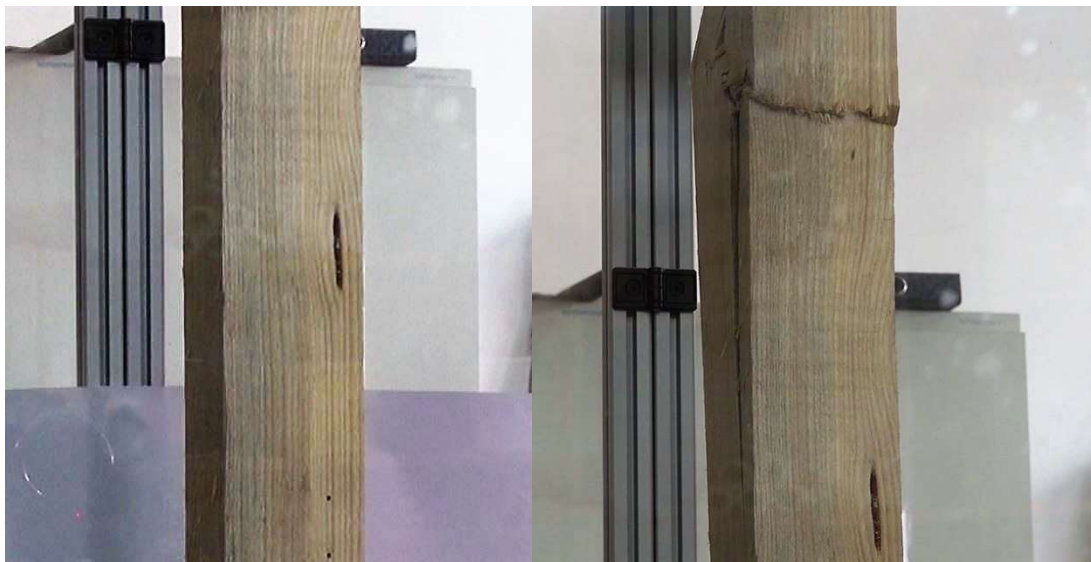
Photo 5-26 Column BN test of load bearing capacity
