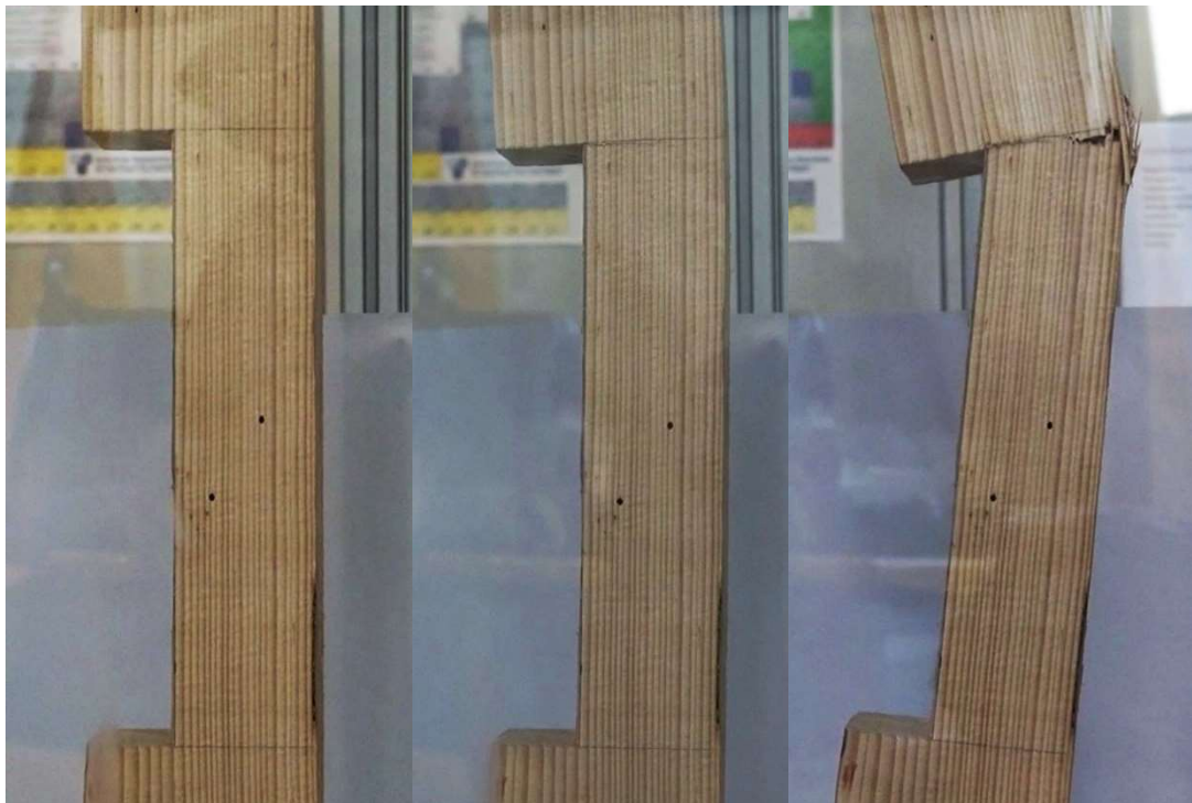
Photo 5–41 Column BD test of load bearing capacity
