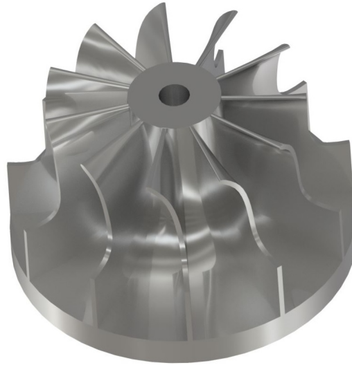
Figure 4.7: 3D model of the impeller of the centrifugal compressor.
