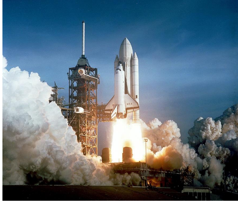
Figure 2 - Space Shuttle Columbia, assigned to mission STS-1, moments after lift-off from Pad 39A, Cape Canaveral, Florida on April 12th, 1981. The two SRBs (Solid Rocket Boosters) are attached to the large external fuel tank, one on each side. [48]
