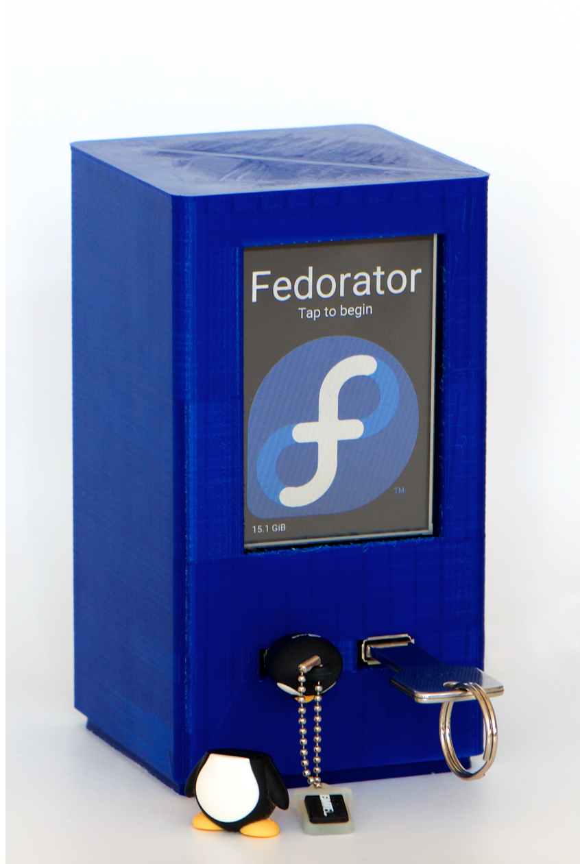
Figure 4.9: The Fedorator prototype with two USB flash drives plugged in
