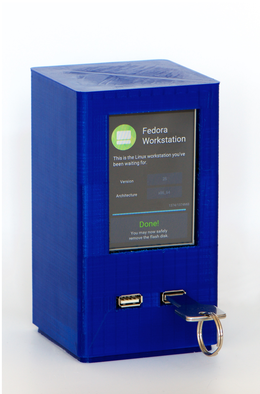
Figure 4.10: The Fedorator prototype done flashing the Fedora Workstation system
