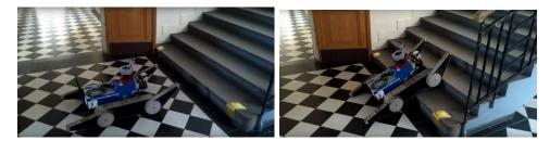
Figure 6.20: Test drive up the stairs
