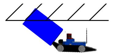
Figure 7.1: Bumper under low ceiling
