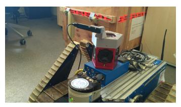
Figure 5.1: RealSense mount
