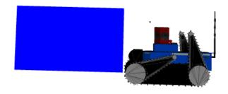
Figure 3.2: Bumper when flippers are up
