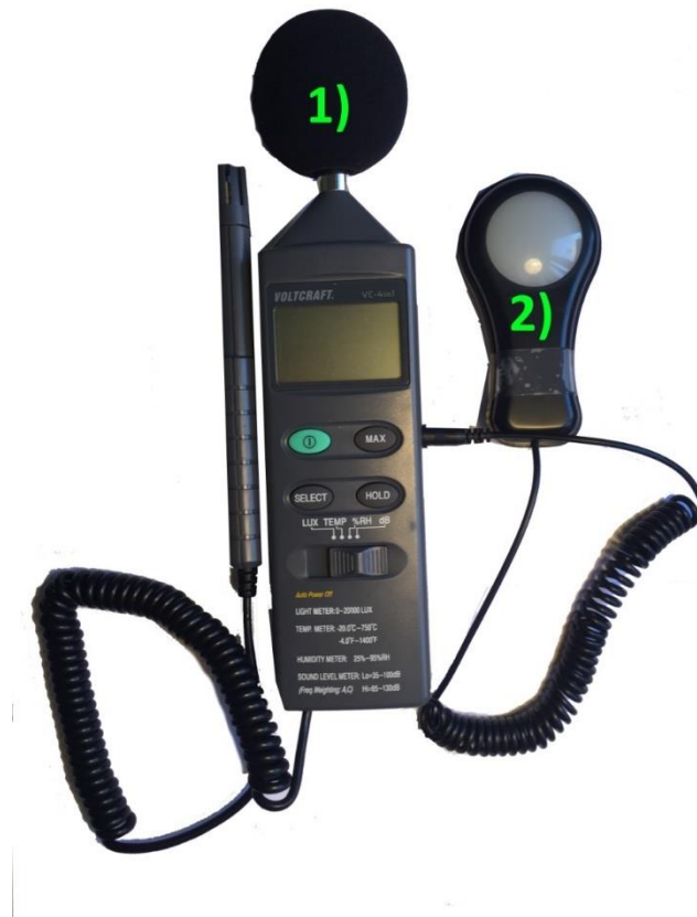
Figure 19: DT-8820 device (1 - sensitive microphone, 2 - photodetector device)
