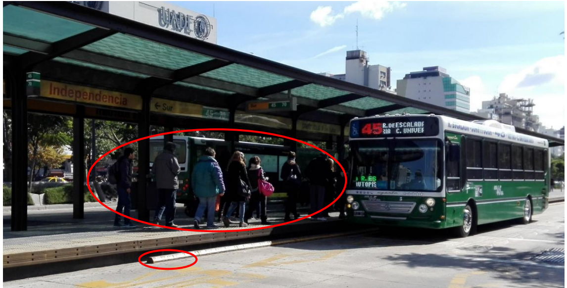
Fig. 18: Station Independencia – queue at the front door; Yellow curbs along the station for reducing the gap between the bus floor and the station platform
