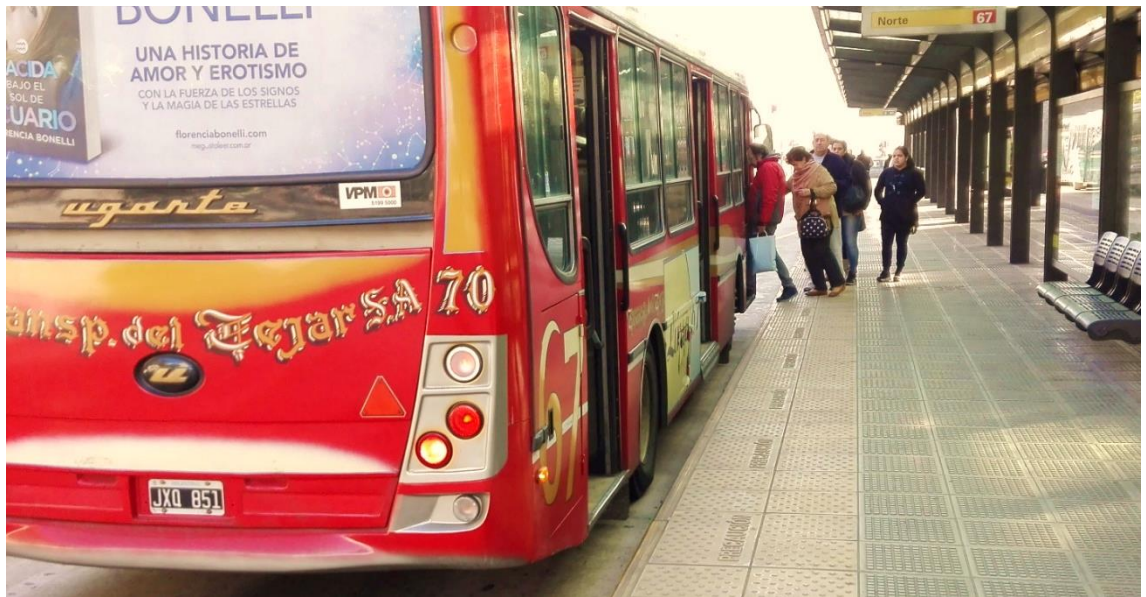
Fig. 28: Bus did not dock properly and has a slight gap between the bus floor and the station platform
