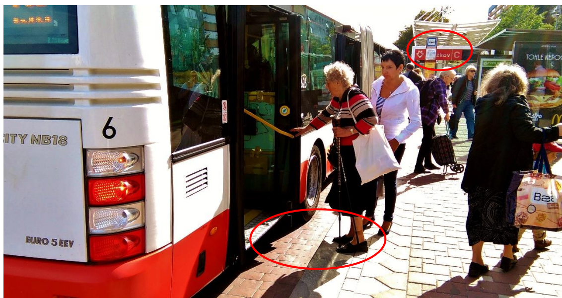
Fig. 63: Larger gap between the bus floor and the stop platform – more difficult boarding and alighting for elderly passengers; in the back of the picture, there is an entrance to the metro station (integration with metro line C)
