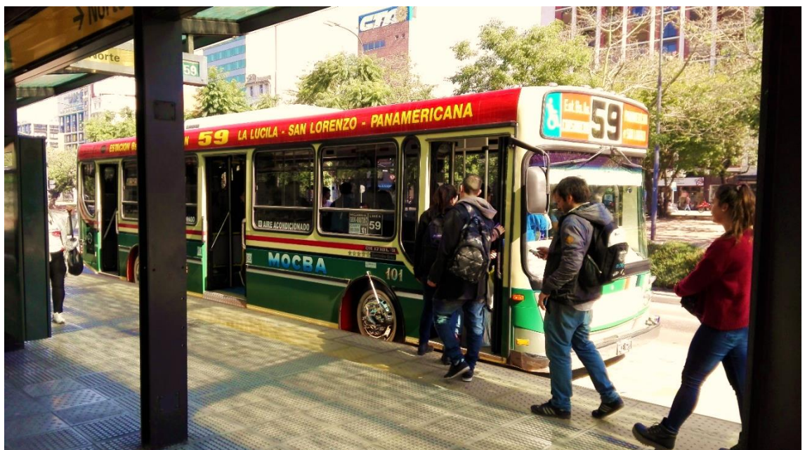
Fig. 22: Regular (non-articulated) bus with 3 doors; Boarding of passengers possible only by the front door
