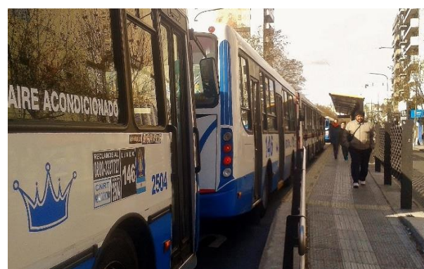
Fig. 36: Queues of buses at stations caused by the absence of passing lanes
