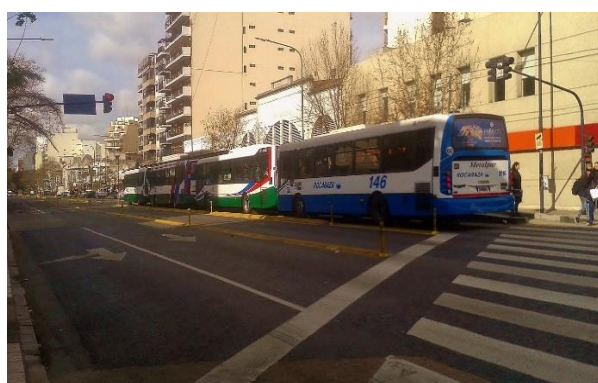
Fig. 36: Queues of buses at stations caused by the absence of passing lanes
