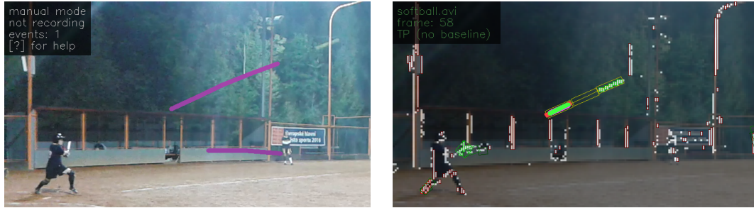
Figure 4.3. Screen captures of the desktop front end. Left: demonstration mode, highlighting detected object traces, and allowing to capture videos. Right: development mode, showing a detailed visualization of the detection procedure.
