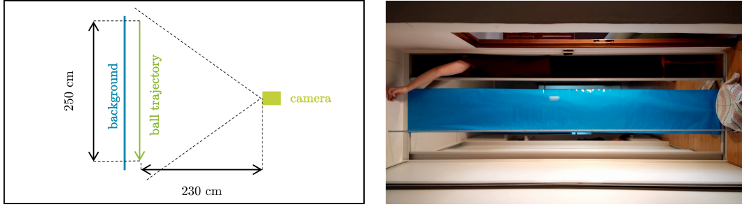
Figure 7.2. Capturing the video sequence for the experiment described in section 7.2. Left: used layout. Right: a typical frame from the captured sequence. The camera is rotated 90 degrees.
