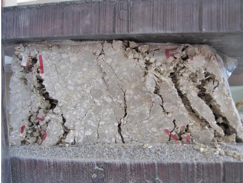
4.2. Breaking of a block belonging to the E + 0.5C + 0.75S -mixture. [12].
