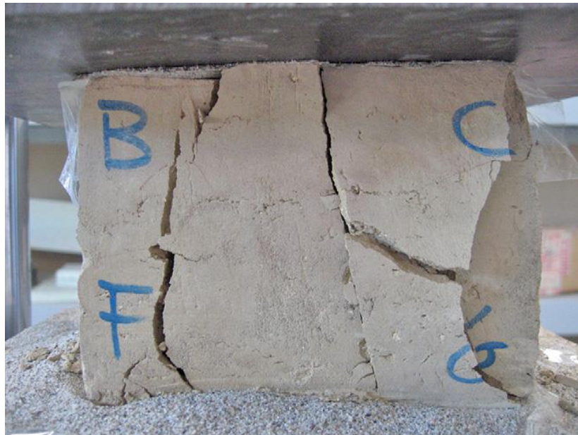
4.1. Breaking of a block belonging to the E-mixture (only earth). Cracks of this mixture typology were punctual and of large size [12].
