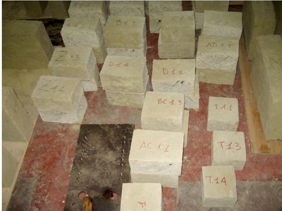
3.8. Sun dried Adobe bricks for the experiment [12]
