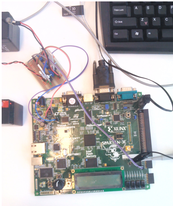
Figure 5.6: FPGA board powered by accumulators, which are connected through stabilizers
