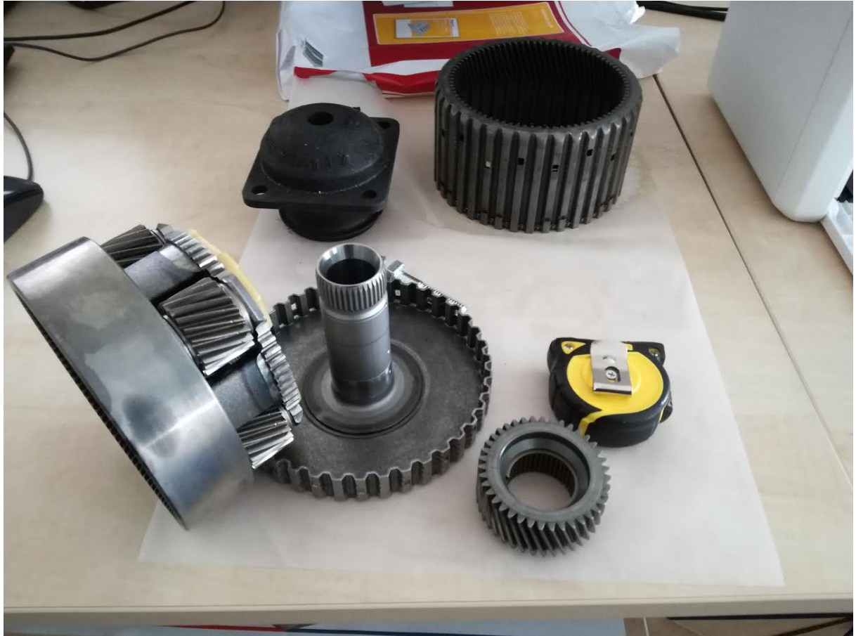
Photo 1 – Planetary gear set elements
