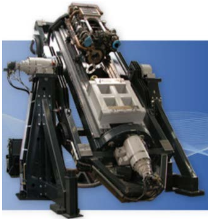
Figure 1.1 – An example of an engine tilting stand, CFM-Schiller, Engine Tilting Test Rig, 2016
