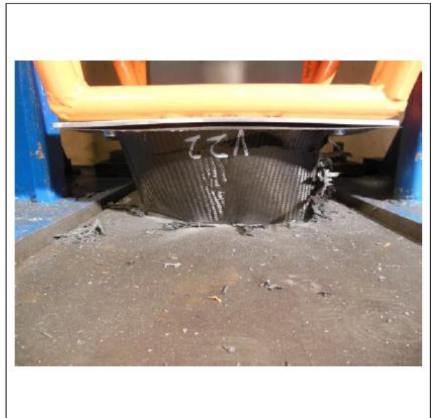
Figure 4: Attenuator after Impact
