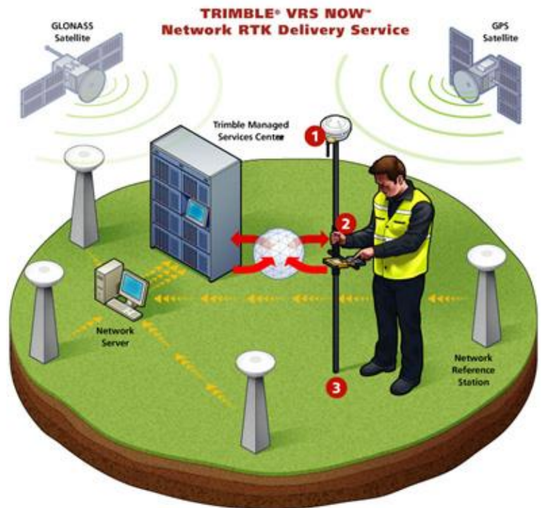
Obr. 14: Princip RTK metody
