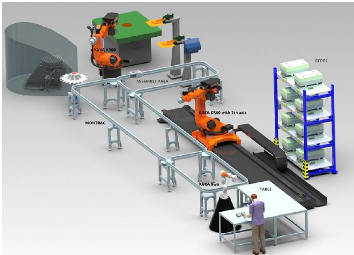
Figure 5.1: Testbed implemented in Process Simulate
