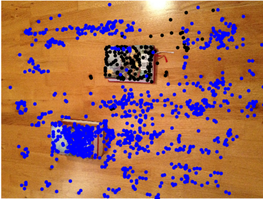
Figure 10: Experiment 3 resulting models. Blue is the background merged with the static bookpile, while the black model is the segmented moving object.
