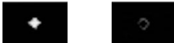
Figure 3.8. The response of a network trained on a binary response map (left) and its error when compared to ground truth (right). The ring in the left image corresponds to the steep change in the error, which is undesired.
