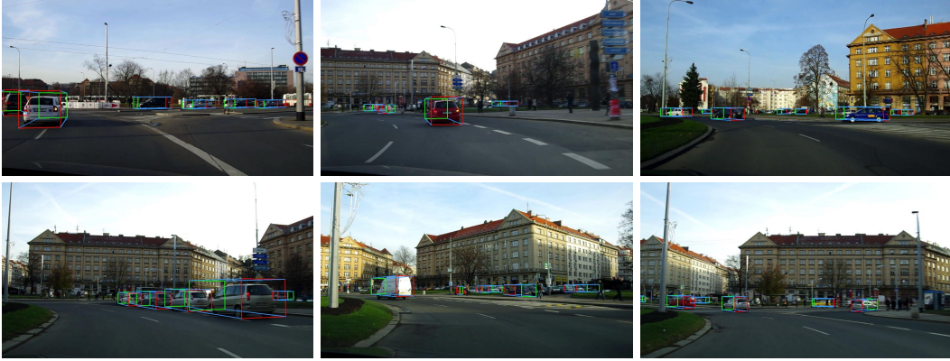
Figure 5.19. Sample images from the Jura test set with the 3D bounding boxes from our best r2_x2_to_x16_s2 network. Only detections with confidence \geq 0.7 .
