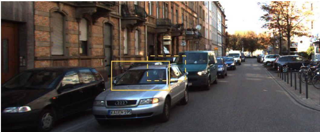
Figure 4.1. An object that according to the methodology should be labeled (solid) vs. object that should not be labeled (dashed). A car from which we would only see a small part of the roof (dashed) would be labeled as don't know since the labeler cannot distinguish whether it actually is a car or some obstacle next to the road. This applies even if the labeler has a prior knowledge from a sequence of images that it actually is a roof of a car.
