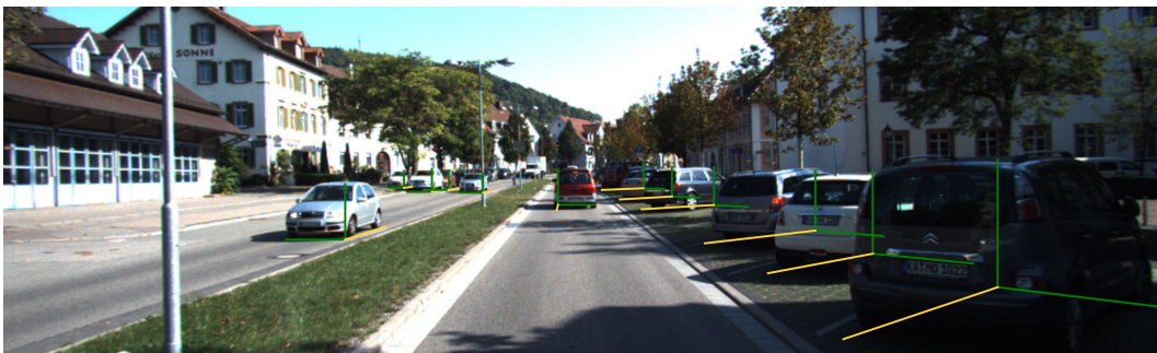
Figure 4.5. Information stored about 3D bounding boxes. Each bounding box is defined by 7 coordinates (3 lines) - front-bottom (green), left-bottom (yellow), front-left (green).
