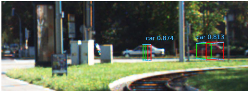
Figure 6.3. 3D bounding box detection with unsure pose. The detector is unsure whether the cars are facing left or right, and hence outputs the average coordinates of the 3D bounding box which is a nonsense.
