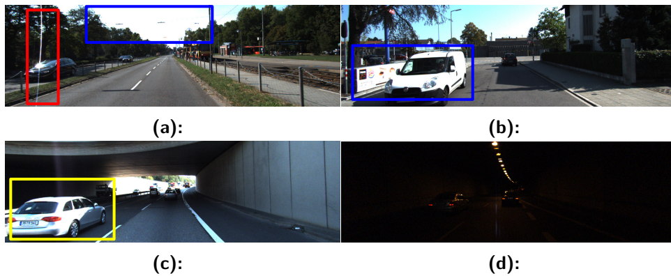
Figure 2.5: Various illumination conditions. Images (a) and (b) show oversaturated areas in the images within blue bounding boxes and reflection in the red bounding box. Image (c) shows strong brightness changes when the car goes to a bridge shadow. Image (d) shows driving during the night with low light. Images are from [MG15].
