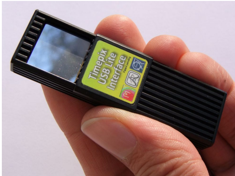
Figure 2 Particle detector Timepix in the smallest variant USB Lite. The Silicon detector chip can be seen on the left (silver surface), the readout electronics is covered by a plastic casing. It is worth noting, that the size of the Silicon chip is the same for all variants at 1.4 \times 1.4 cm. Source: http://aladdin.utef.cvut.cz/utef_web_pictures/anniversary/tpx_usb_lite_small.jpg
