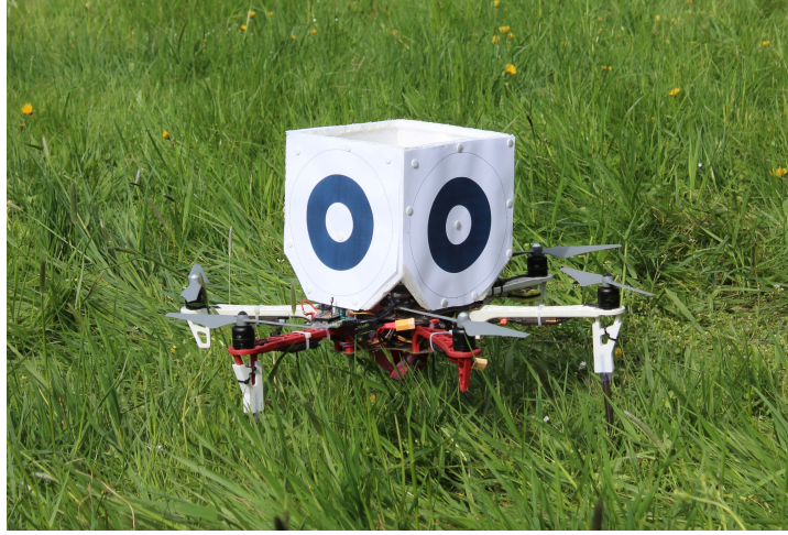
Figure 25 The pattern used for relative visual onboard localization by the MRS group.
