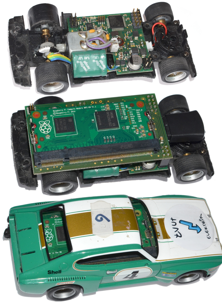
Figure 2.1: The hardware of the car; the bottom board, the top board, and the car.
