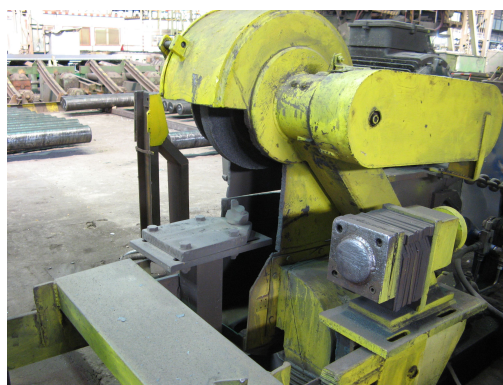
Figure 2.3: Current grinding station [2]
