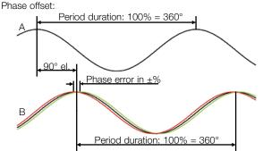
El. phase offset:  $90^{\circ} \pm max$ . phase error 7,5% of a pulse length
