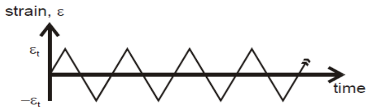
Figure 3. 5: Constant Strain Amplitude load history
