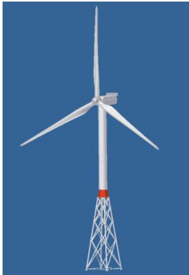
Figure 2.13: CAD model of hybrid lattice-tubular wind turbine with transition segment (Bremerhaven prototype) [7]
