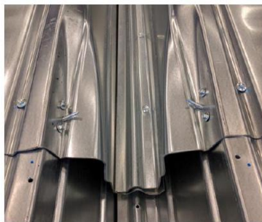
Figure 3.15 Local Web Buckling of LHP200, t=1.50\text{mm}
