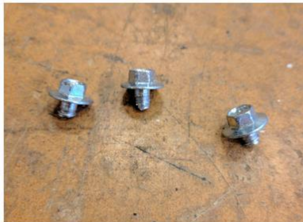
Figure 3.16 Tensile Failure of the Side-Overlap Connection Screws, LHP200, t=1.50mm
