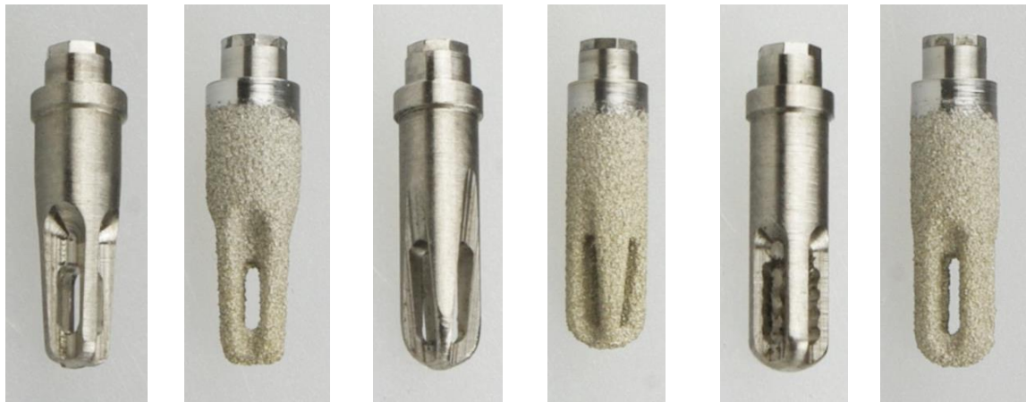
Fig. 21: Manufactured functional titanium implant stems coated with porous titanium by means of plasma spraying. Conical stem with oblique beams (left), cylindrical stem with oblique beams (middle) and cylindrical stem with parallel beams (right). Images obtained from the 2015 TA03010886 project report submitted by CTU Prague, Faculty of Civil Engineering.
