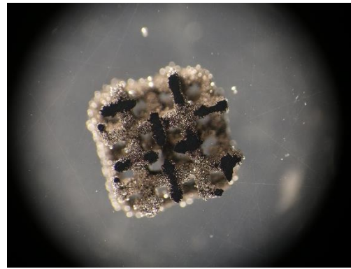
b) trabecular cross-section of an implant test specimen
