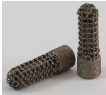
a) whole implant body, consisting of both the trabecular and homogeneous structure
