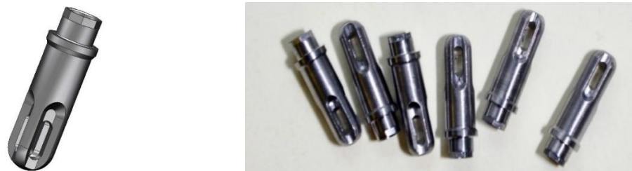
Fig. 18: Figures showing geometrically modified Ti-6Al-4V ELI (extra-low interstitial) implants. Geometrical model (left) and cylinder-shaped implants with parallel beams (right).
