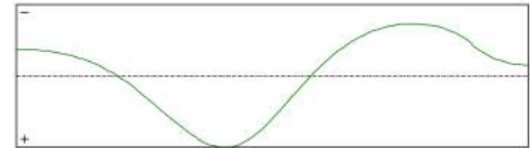
Figure 8 : Warping component of the shear centre (Mode 1).
