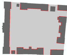
(a) Ratio of borders of open space (light gray) to borders shared with enclosing buildings (red) is 0.84. Source: author
