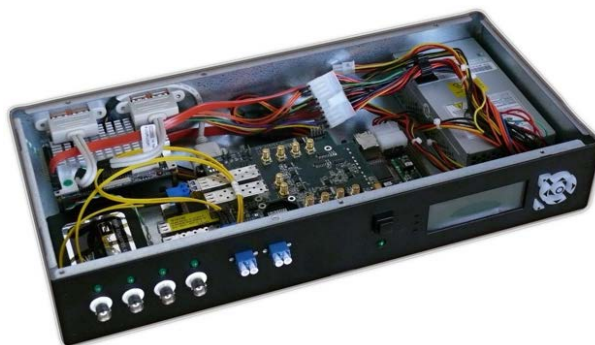
Figure 30: Working sample of a two-way time transfer adapter
