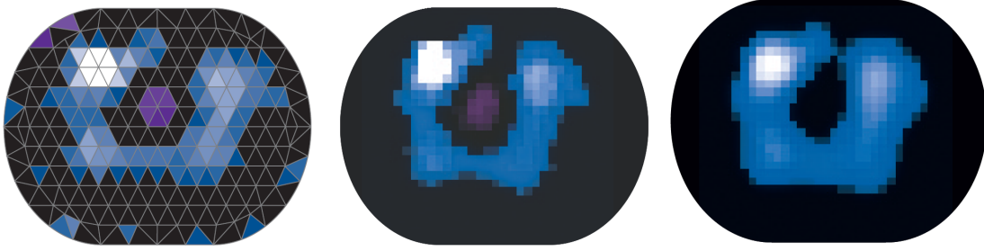
Figure 1.3: Transformation of triangular mesh into EIT image. Left: the values of relative impedance are assigned to triangular elements. Middle: triangular mesh is co-registered into rectangular elements and the artefacts that are close to the boundary are damped. Right: a Gaussian filter is used to smooth the image. Adopted from [17].
