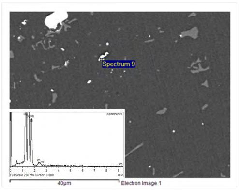
FIGURE 5. The EDX analysis of the aluminium alloy after ECAP and heat treatment.
