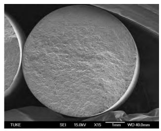
FIGURE 10. The fracture surface of EN AW 6012 in the post-ECAP state.
