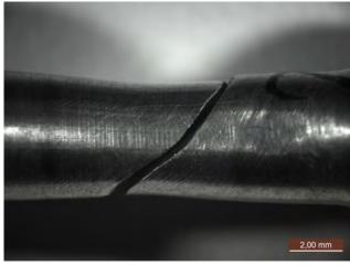
FIGURE 8. Fracture of EN AW 6012 alloy post-ECAP.
