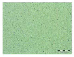
FIGURE 2. Microstructure of the aluminium alloy in the initial state.
