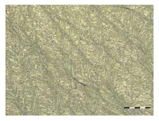
FIGURE 3. Microstructure of the aluminium alloy after ECAP and heat treatment.
