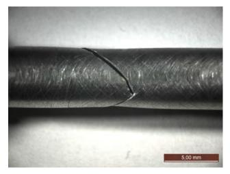
FIGURE 7. Fracture of EN AW 6012 alloy in pre-ECAP.
