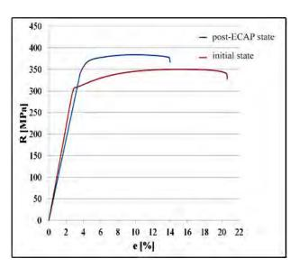
FIGURE 6. Dependent force of strain and elongation in the static condition of EN AW6012.
