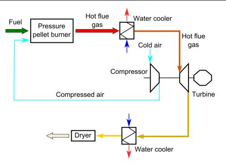
FIGURE 2. Scheme of the technology — Solution 6.
