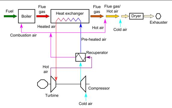
FIGURE 1. Scheme of the designed technology — Solution 1.
