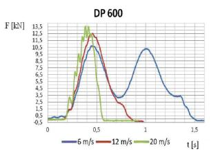
FIGURE 9. Dynamic tensile curves of DP steel.
