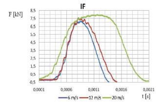
FIGURE 8. Dynamic tensile curves of IF steel.
