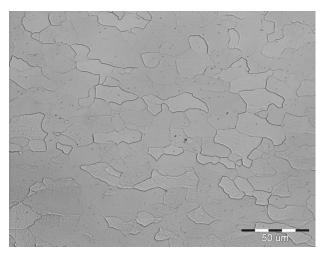
FIGURE 2. Microstructure of IF steel.
