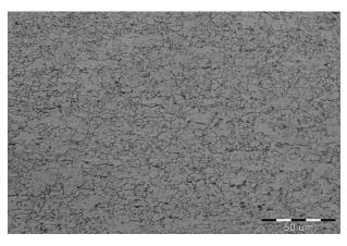
FIGURE 4. Microstructure of HSLA steel.
