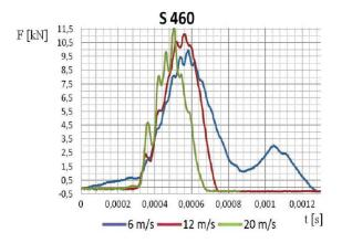
FIGURE 10. Dynamic tensile curves of S 460 steel.
