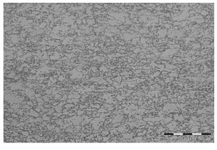
FIGURE 3. Microstructure of DP steel.
